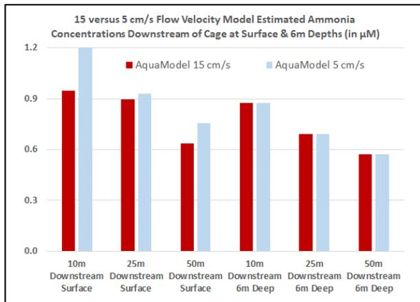
**Figure 12. Graphic comparison of AquaModel estimated ammonia concentrations downstream of cage at 15 versus 5 cm sec<sup>-1</sup>.**
