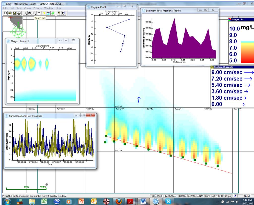
**Figure 1. Example of eleven fish cages in British Columbia showing oxygen reduction and recovery downstream along with current velocity record being used and a plot of sediment organic carbon effects<sup>1/</sup>**
