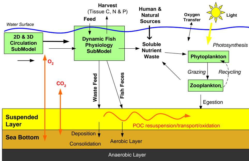
**Figure 2. Conceptual water column and benthic interactions within AquaModel software.**
