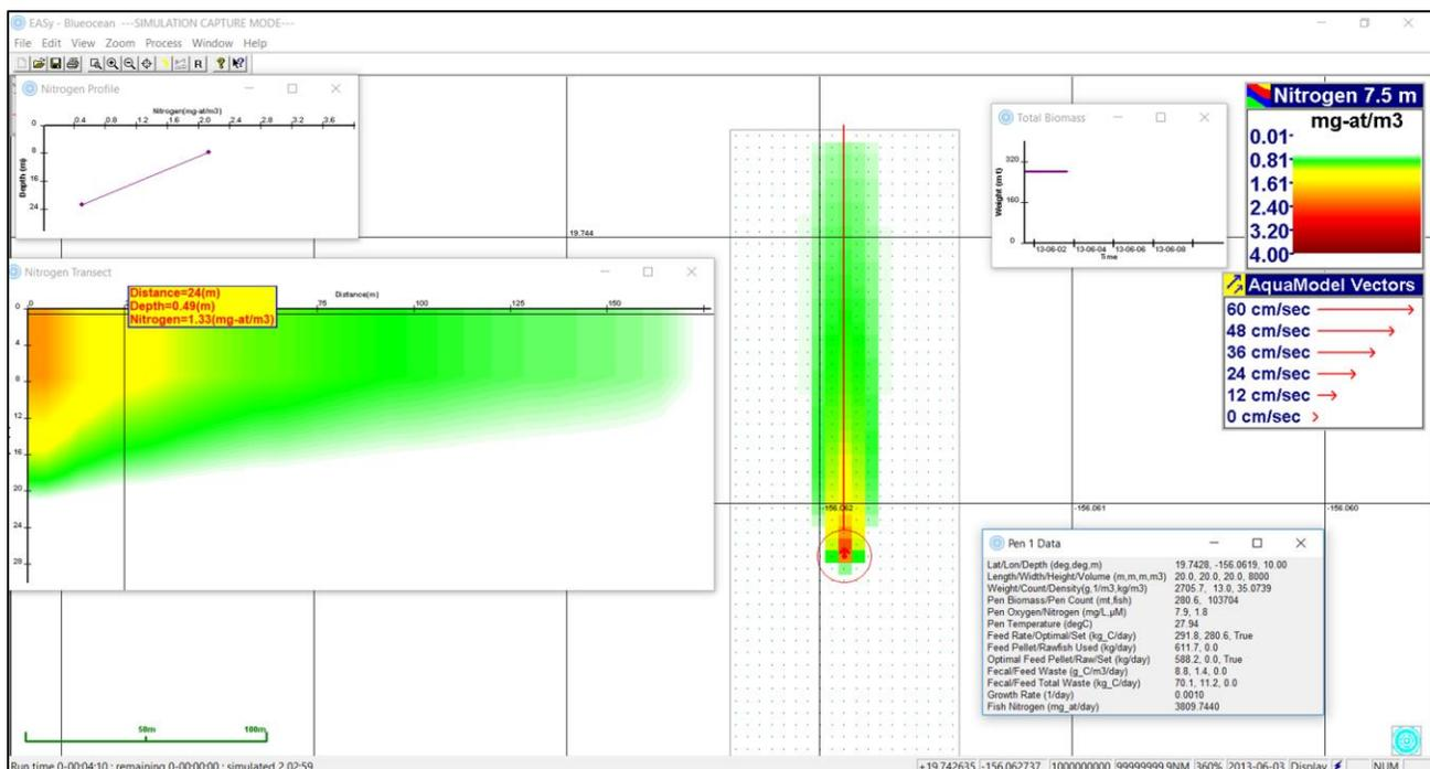
Figure 11. AquaModel screen print showing plan (center) and side profile plot (left side) of the simulation in process using a steady current velocity of 2 cm sec<sup>-1</sup> displaying total dissolved nitrogen in μM units.
