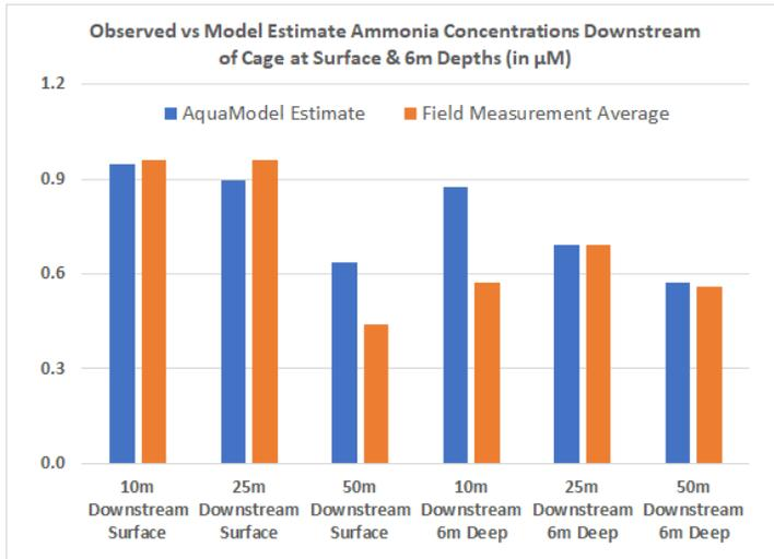
**Figure 10. Observed versus AquaModel estimated water column nitrogen distribution from the studied net pen.**
