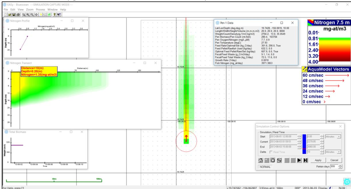
Figure 9. AquaModel screen print showing plan (center) and side profile plot (left side) of the simulation in process using a steady current velocity of 15 cm sec<sup>-1</sup>.
