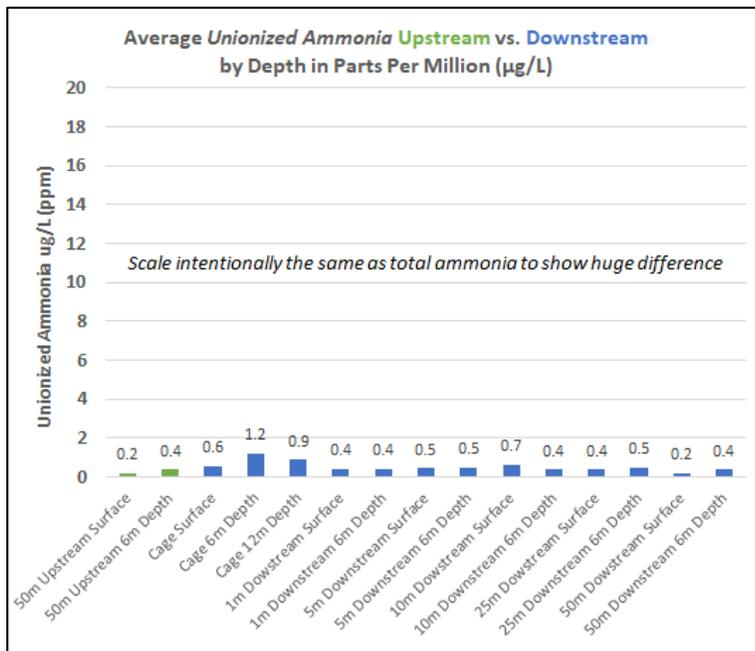
**Figure 8. Un-ionized (potentially toxic) ammonia concentration estimates from field work measurements.**
