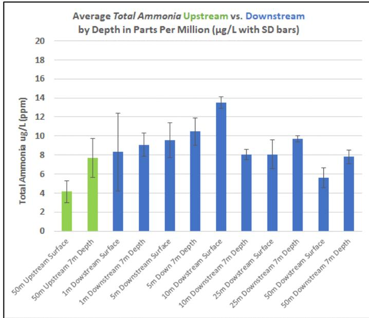
Figure 6. Average total ammonia at sampling location with one standard deviation error bars.
